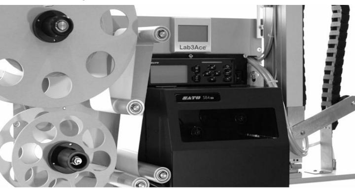
**In-Line Print & Apply** system with fast and accurate application of labels in the production line, that keeps label wastage to the absolute minimum. This applicator is designed to apply the label either on top, bottom, or side of the product. It operates if the product are moving or stationary. The machine's special characteristics are robustness, speed, flexibility and small footprint.
